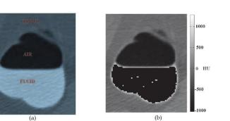
**Figure 1**: 2D slices of: a) 3D CT data; b) 3D CT data after classical thresholding operation.
