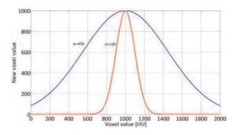
**Figure 5**: Gaussian transfer functions; blue line – for fluid mask  $\sigma$ =450, red line – for residual mask  $\sigma$ =100.
